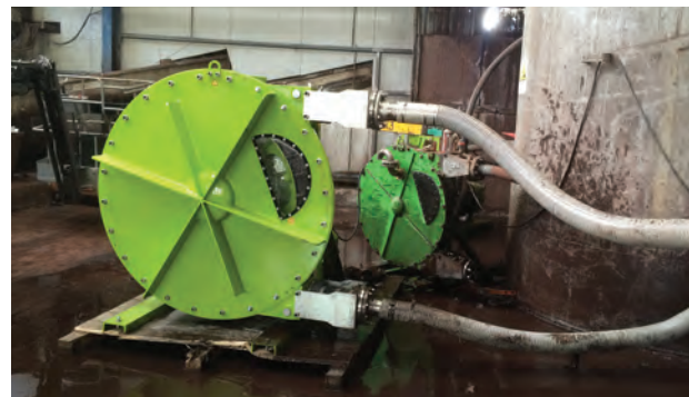
ALH125 for car battery recycling, handling wastewater and slurries
