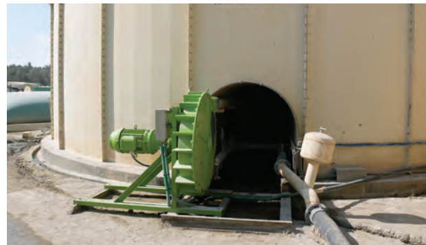
ALH100 pumping thickener underflow in a quarry
